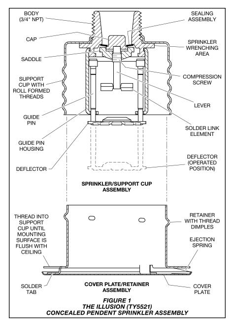
current NFPA standard; however, in accordance with its UL and C-UL Listing it cannot be used for the protection of storage.
